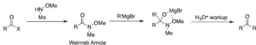
Fig . The preparation of Weinreb amide from carboxylic acid derivatives and its reaction with Grignard reagent.
