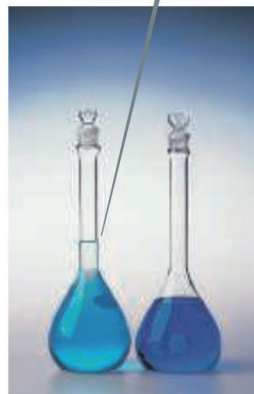
Preparing 250.0 mL of 0.100 M \text{CuSO}_4 by dilution of 1.00 M \text{CuSO}_4 .
