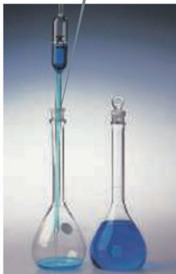
Preparing 250.0 mL of 0.100 M \text{CuSO}_4 by dilution of 1.00 M \text{CuSO}_4 .
