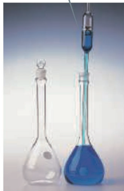
Preparing 250.0 mL of 0.100 M \text{CuSO}_4 by dilution of 1.00 M \text{CuSO}_4 .
